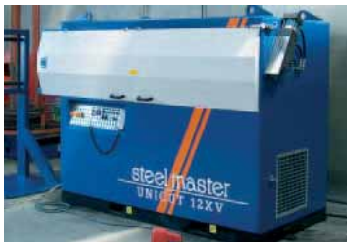
UNICUT 12XV for straightening- and cutting coil from Ø 6 to 12 mm (#2-4).
