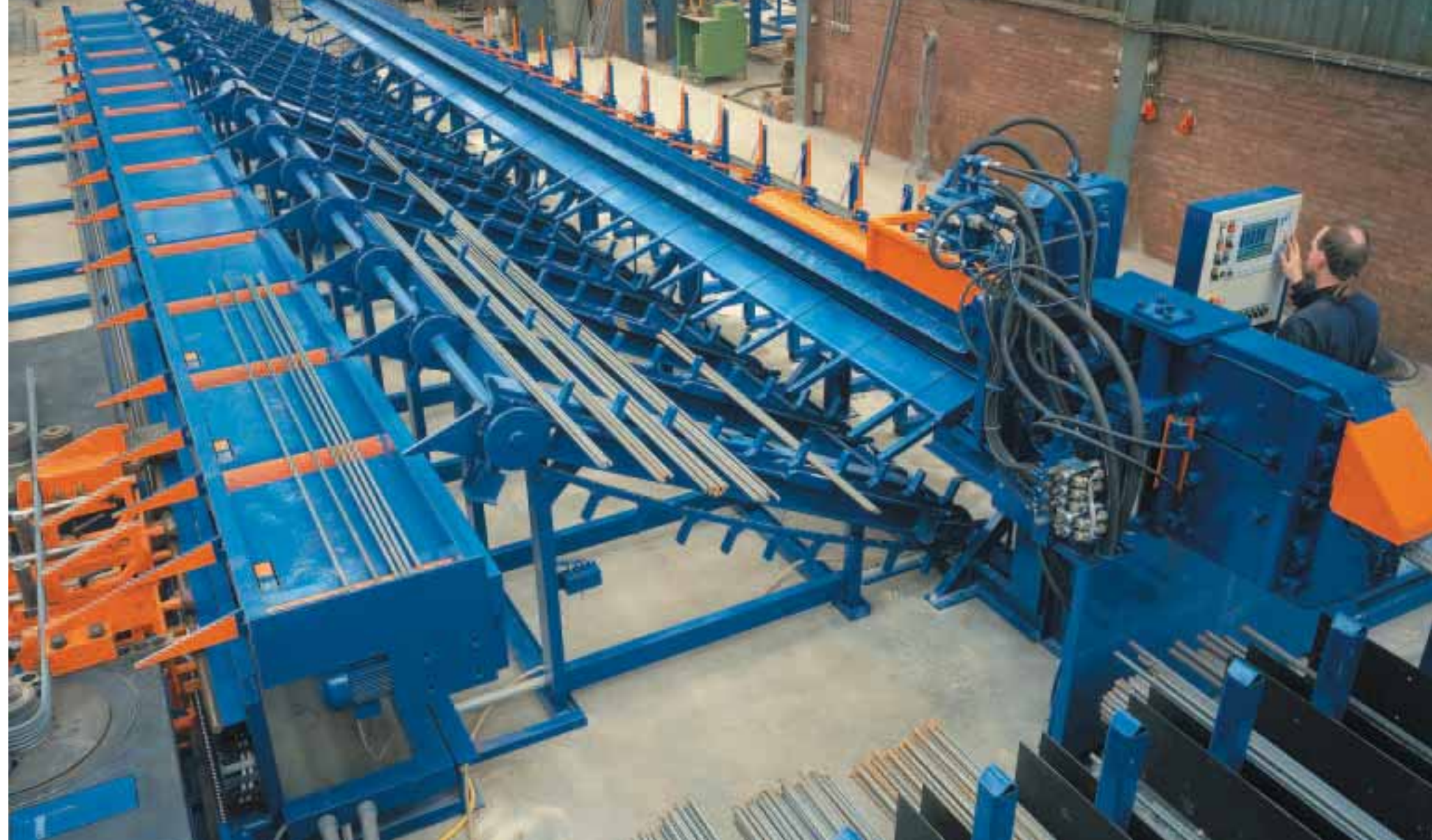
Combine bar shearing and bending line.
